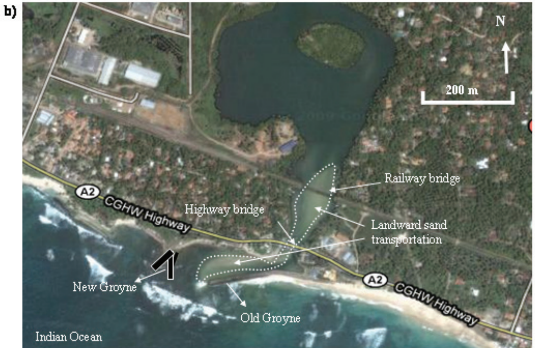
Figure 16.2 a) Satellite image of Koggala lagoon outlet with sand bar and manually cut opening in 1985 (Source: Coast Conservation Department, SL); b) Satellite image of lagoon outlet with the existing groyne structures.
