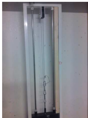
Figure 5: Locking device, used during the isometric measurements.
