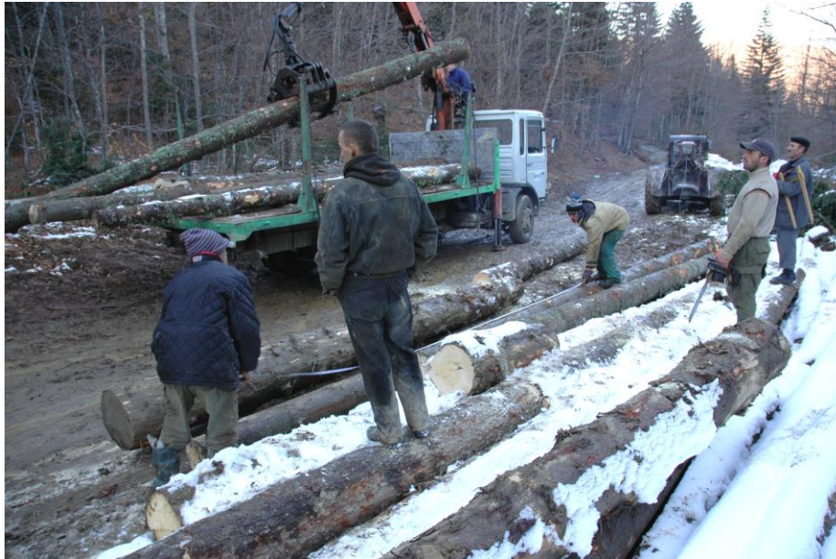
Loading the truck prior to the road transport. The logs are measured before loading.
