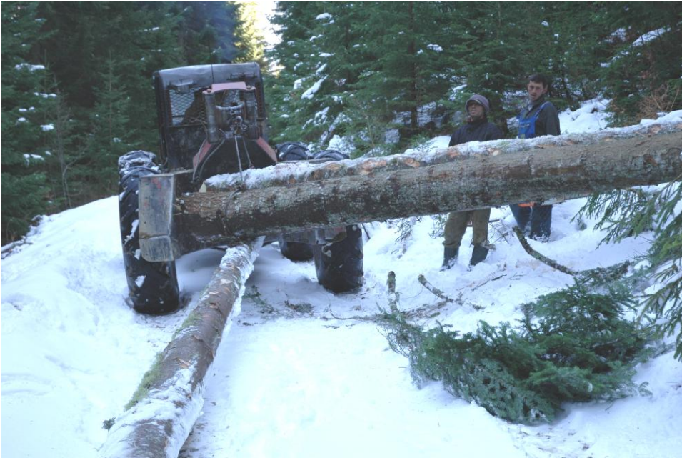
A Timberjack skidder is used for the terrain transport of logs.
