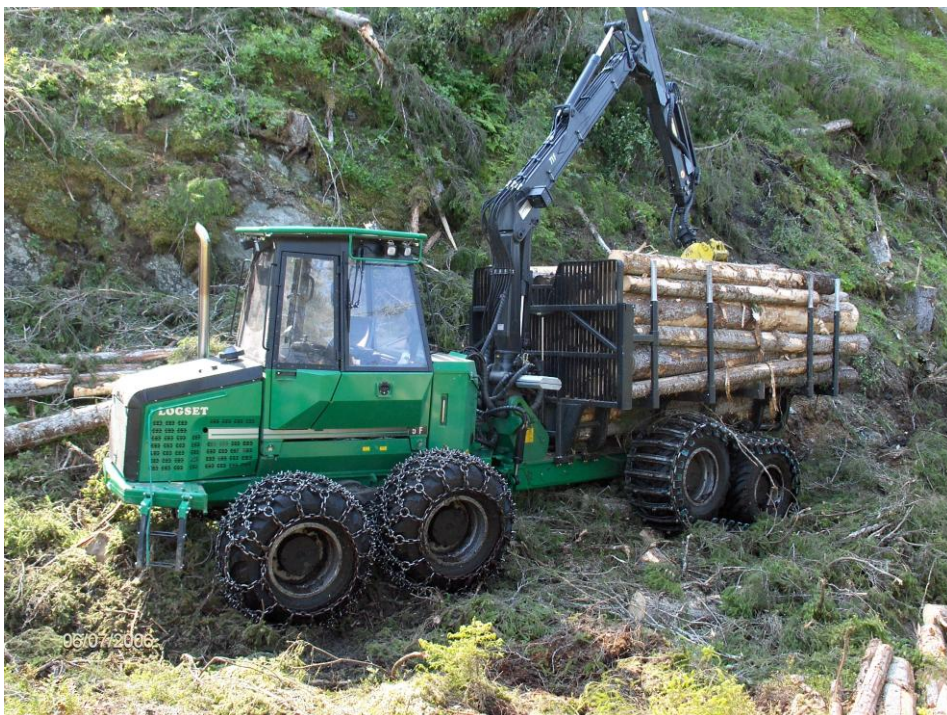
Logset forwarder with 8 wheel drive for terrain transport
