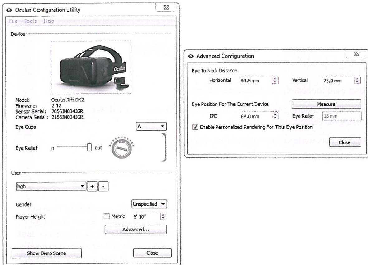
Figure 8: Private screenshot of the settings used. As shown, Oculus VR use the population average IPD of 64mm as default (3.2.2 Interpupillary distance).
