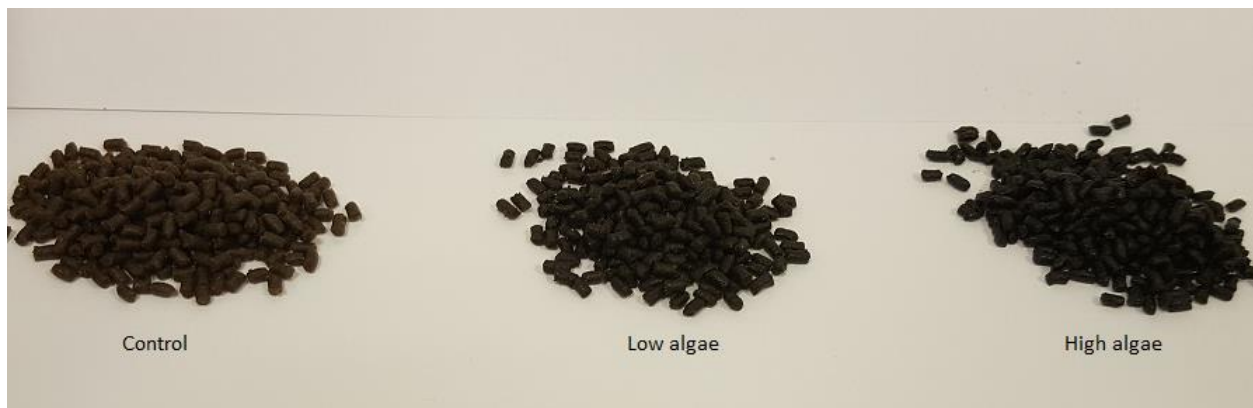
Figure 8. Visual appearance of the experimental diet after extruder. The color of the control diet was light brown and become light green in low algae and dark green in high algae.
