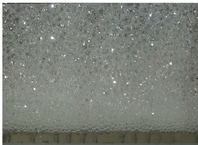
Fig. 3. Liquid fraction gradient in a rising foam column, without applying liquid recirculation. The liquid fraction of the foam is high at the bottom of the foam column, close to the foam-liquid interface, while it is decreasing towards the top foam layers.
