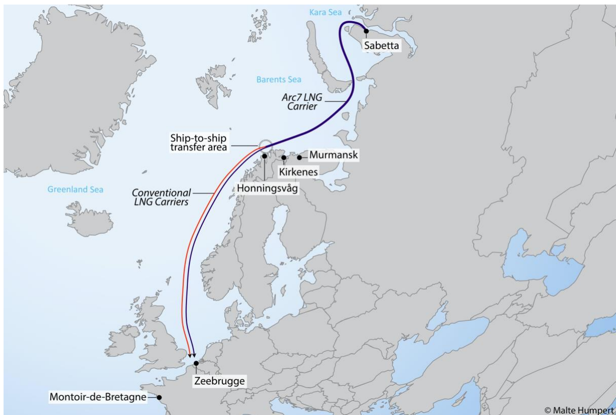
Map 4.2: Map showing Novatek's winter operation delivering LNG from Sabetta to Europe onboard Arc7 carriers or conventional carriers after ship-to-ship transfer off northern Norway (Humpert, 2020)
