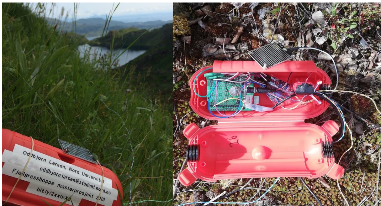
Figure 2 The sensor box, on the left side is a sensor box placed in a habitat without grasshoppers, the rain sensor can be seen on top, and wires going to the soil moisture sensors can be seen in the bottom right corner. On the right is a photo of the inside of a sensor box, where the Arduino low power shield can be seen together with the battery and miscellaneous wires.
