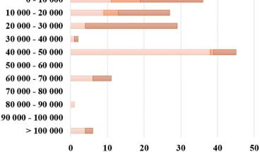
*Figure 3.* Transit voyages on the NSR per vessel gross tonnage (GRT). In 2010–2013 most voyages involved vessels in the 40,000–50,000 GRT range (tankers and bulkers); and 20,000–30,000 GRT in 2016–2019 (general cargo/heavy lift carriers). Data sources: Atomflot (2010–2012) corrected for full transits only, NSRA (2013–2019), CHNL Information Office (2016–2019).
