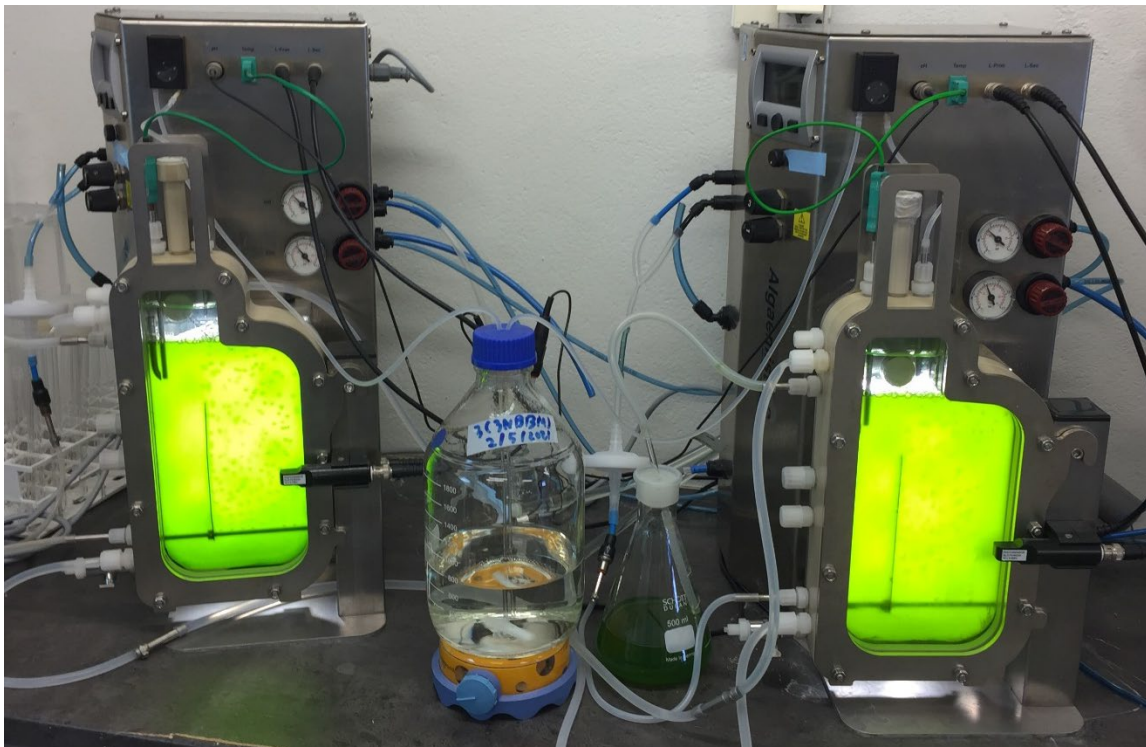
Figure 3. The assembled Algaemist-S flat-panel photobioreactor. 2L bottle in the middle holds the medium. Erlenmeyer flask collects the out-flow from the reactor. Light-blocking covers were temporarily removed in this picture.
