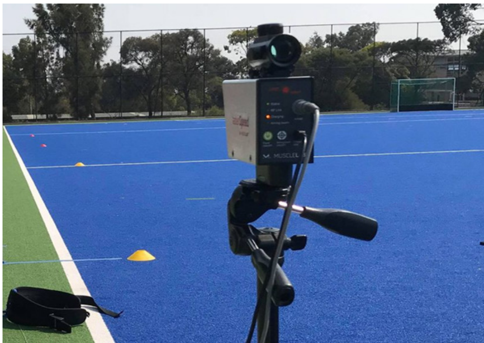
Figure 2. MuscleLab™ is a system which uses an optical laser to measure sprint distance over time and automatically calculates sprint mechanical properties
