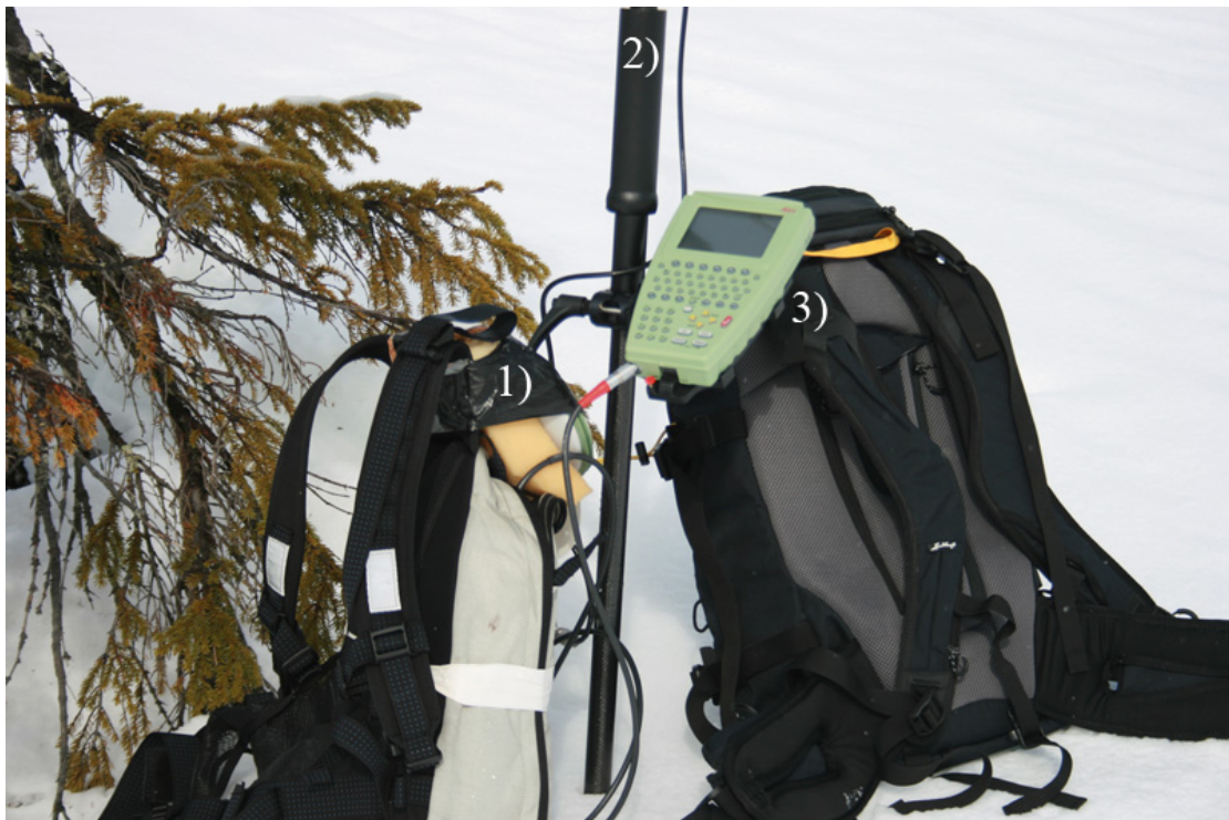
Figure 2. The RTK GNSS system, consisting of: 1) Leica GX1230 GG, 72 channel, dual frequency L1/L2 receivers, 2) Leica AX1202 GG survey antennas and 3) Leica GFU14 Satelline 3AS radio modems (Leica Geosystems AG, Heerbrugg, Switzerland).
