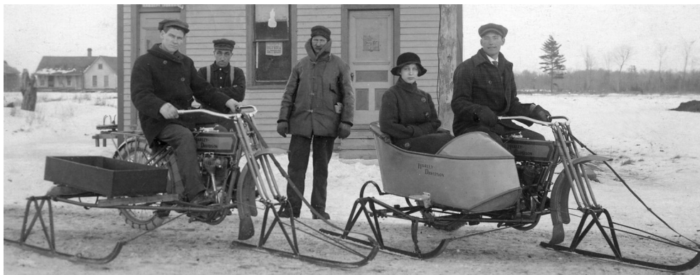
Enlargement of a postcard released in USA showing two Harley Davidson motorcycles converted to use on ice and snow. The rear wheels have chains attached to the standard rubber tires. (Postcard of unknown origin).
