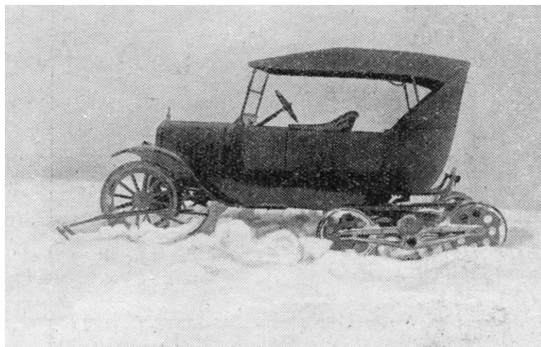
As we see the front wheels were equipped with skis on the front axle making it possible for use in snow and on ice.(Meddelelser fra Veidirektøren Nr. 7, 1925.)
