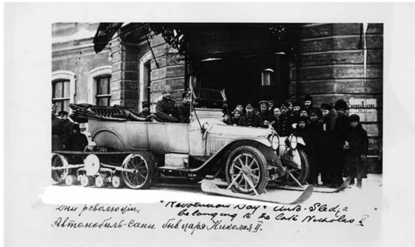
The Kégresse system used on a 1915 Packard 3-38 belonging to Czar Nicolas II (Picture from Detroit Public Library, Item number EB01c673)
