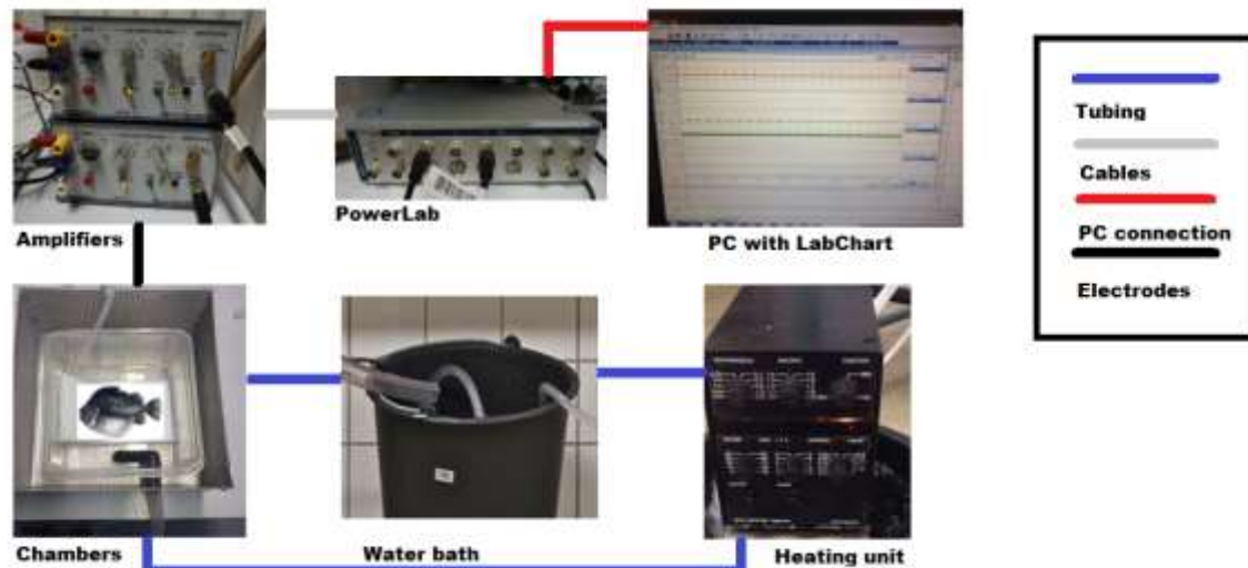
Figure 5. Overview of the experimental set-up, with all parts and their connections. The computer with the LabChart software was connected to the PowerLab unit, which again was connected to amplifiers. Electrodes were extended from the amplifiers to the fish for recording of ECG signals.
