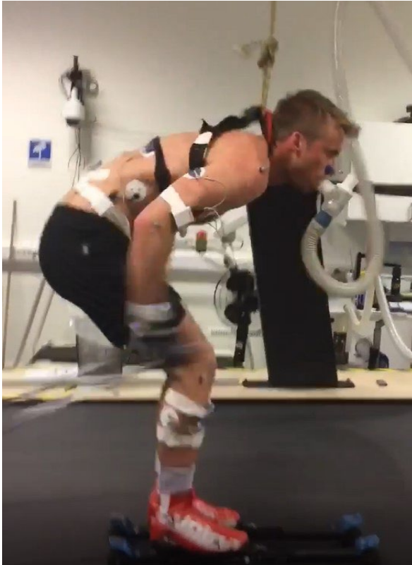
Figure 2: An Olympic distance skier testing gas exchange, kinematics and EMG in the laboratory
