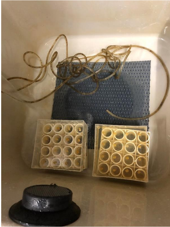
Figure 5. Incubators for egg strings and the planktonic stages of sea lice. The incubators allow for water exchange by allowing filtered seawater to enter slowly through the lid, flow through the 16 chambers, and exit through the mesh bottom of the incubator (Photo: Tuva Sørgaard).
