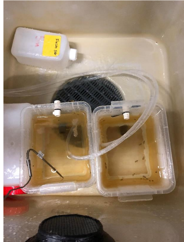
Figure 6. Incubators for the larger life stages of sea lice. The incubators have mesh at the bottom, which allows for water exchange. The two incubators are placed in each level tank, which is a regular container without mesh. Filtered seawater runs through the tubes and into the incubators (Photo: Tuva Sørgaard).
