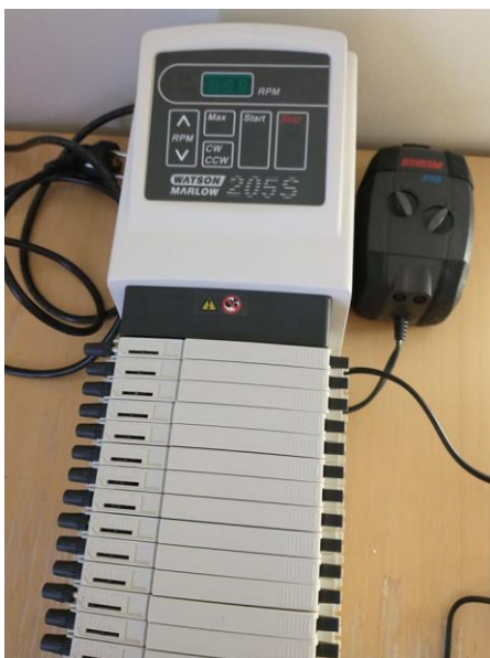
Figure 7 The Watson Marlow 205 series 16-channel 8-roller pump
