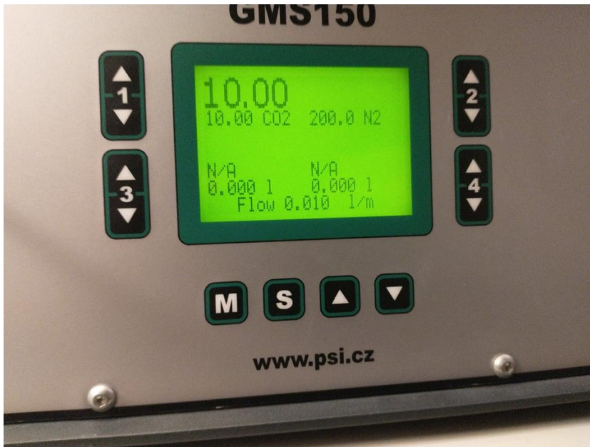
Figure 6 The Gas Mixing System GMS 150 (Photon System Instruments, PSI). Can be tuned to output the desired volume of CO 2 .
