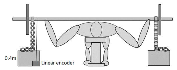
Figure 1. Bench press set up with chains and linear encoder attached to the barbell.
